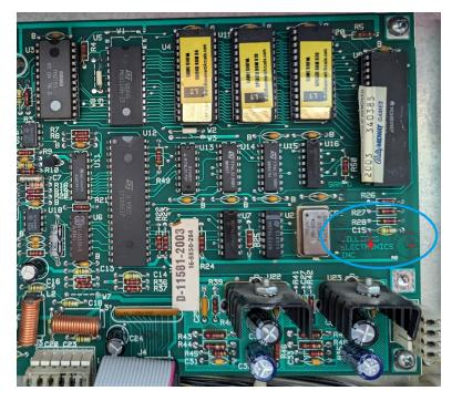
2) Add a jumper from the aux reset test point on the Warped Pinball SYS11. Wifi board to the left side of C15 on the sound board.
