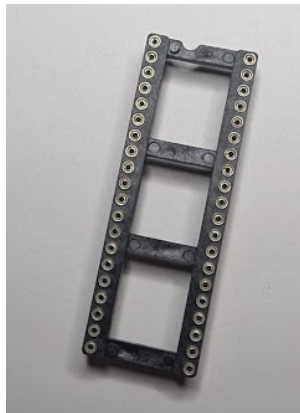
Round pin chip carrier Insert on top of the pin strip headers
