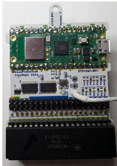
Processor chip inserted into socket on Wapred Pinball SYS11.Wifi
