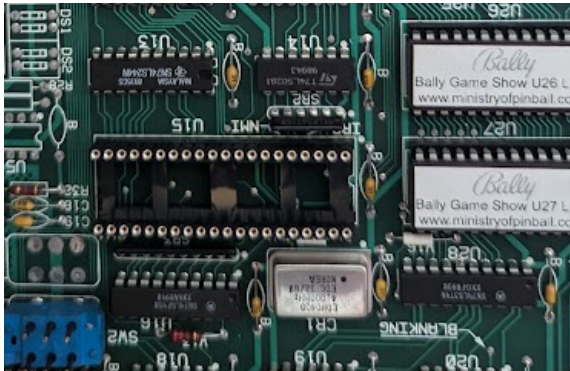
Main processor socket with pin strip header
