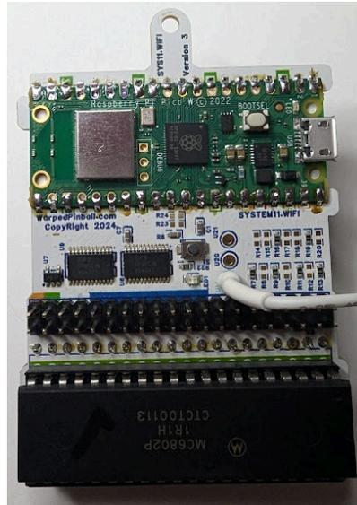
Processor chip inserted into socket on Waped Pinball SYS9.Wifi
